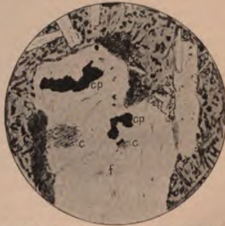
FIG. 7.—NATIVE COPPER, REPLACING FELDSPAR IN TRIASSIC ANDESITE-BASALT, COPPER UNION, COPPER BUTTE DISTRICT. f , FELDSPAR; c , CALCITE; cp , COPPER. (MAGNIFIED 120 DIAMETERS. LINDGREN)
